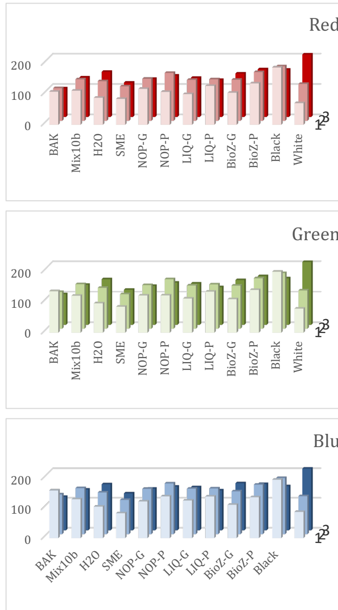
Figure 24. Histograms of the RGB mean values obtained from the photographs rectangular sections related to different exposure times. Black and White are respectively the most darkening and lightening intensity of not treated surface.
